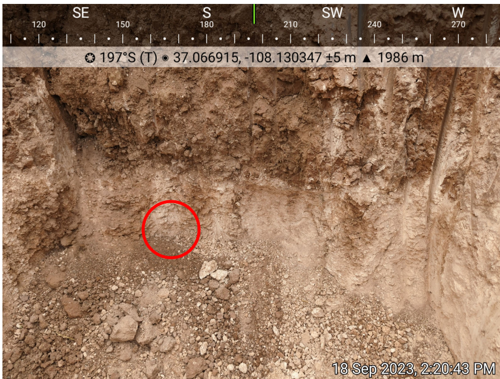
Photo 14: SS12 collected from south sidewall of flowline excavation area, 9/18/2023
