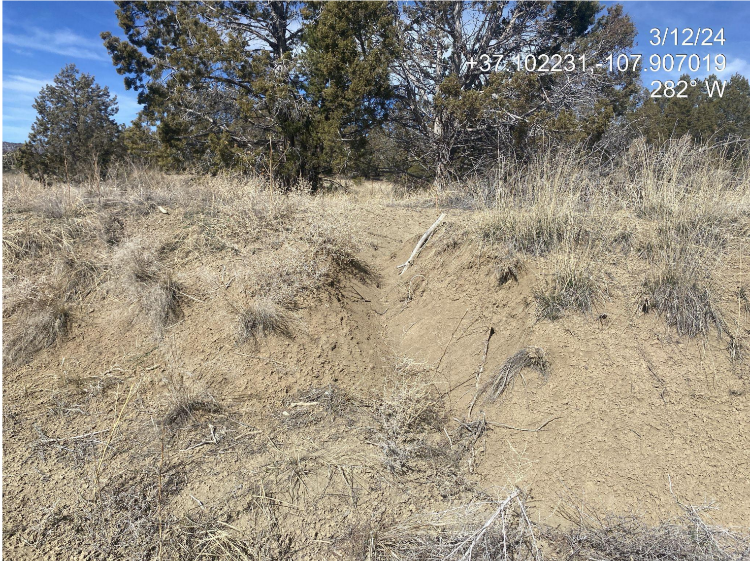
Photo 5. View of gully erosion forming in the western interim reclamation area.
