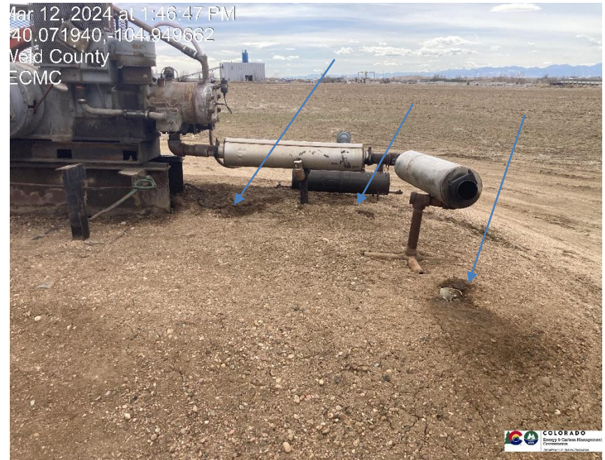
Pic 4 Stained soil / mechanical issue by gas motor
