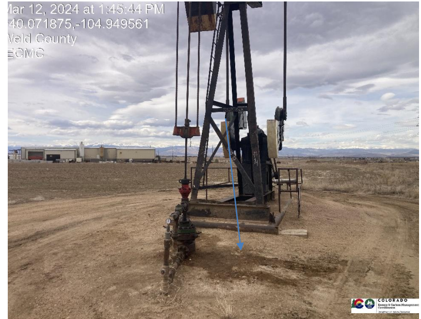
Pic 2 pump jack, stained soil
