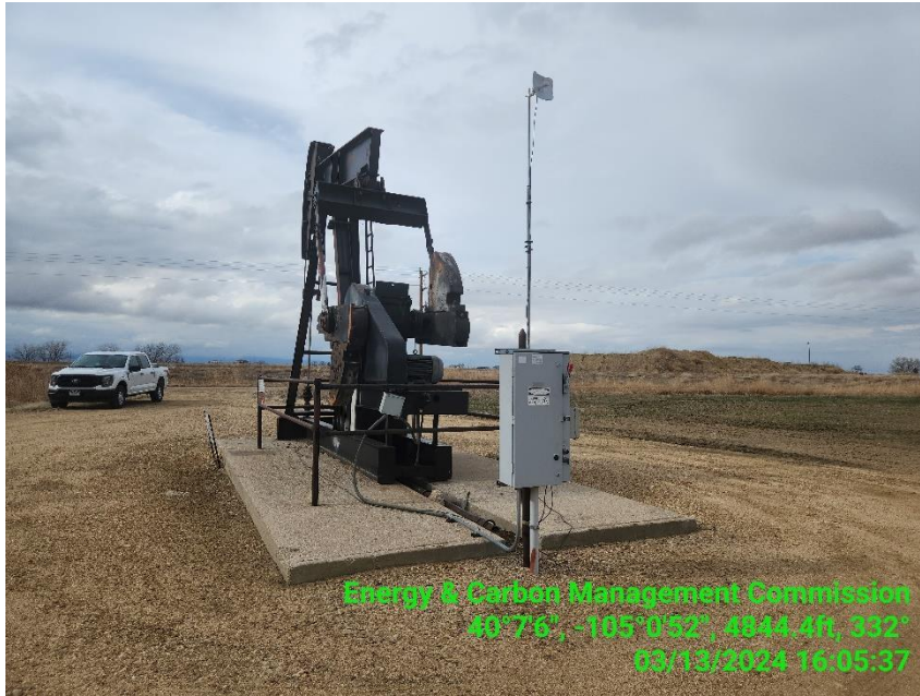
Photo 5 PJ, electric panel & telemetry
