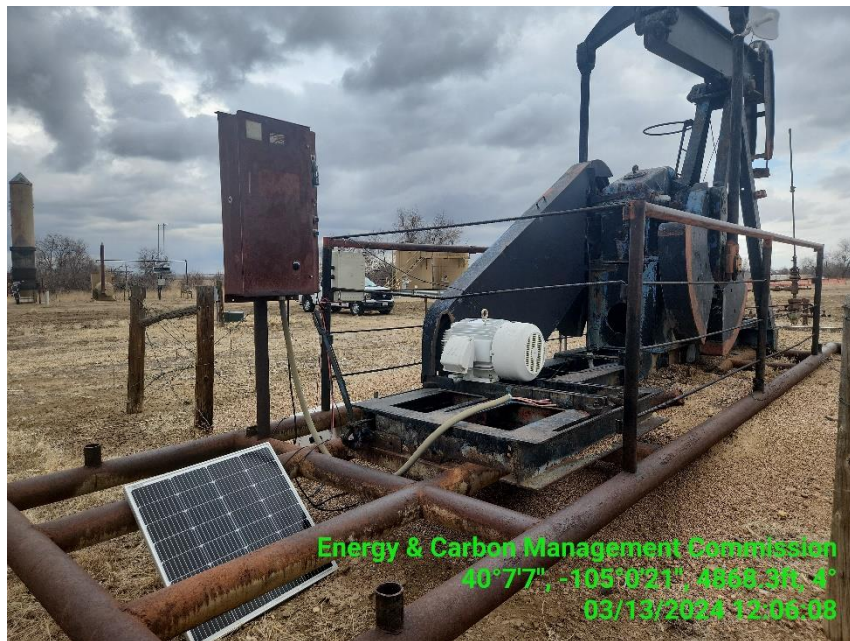
Photo 5 Electric panel for the electric motor is shut off .
