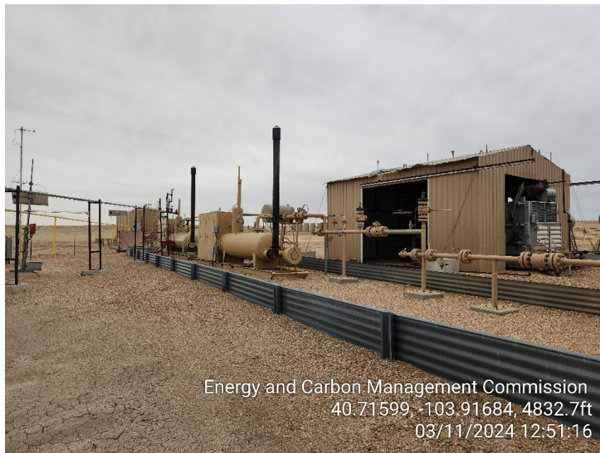
Photo 11 – Separators and Compressor
