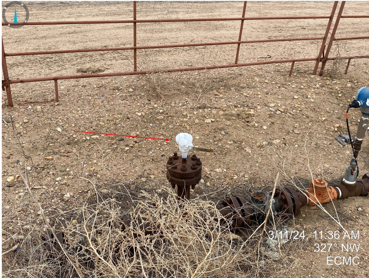
Photo 10. Audible leak and apparent frost accumulation on valve at Well API 123-41883.
