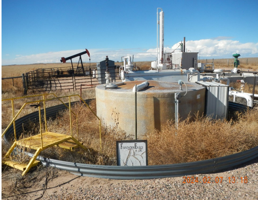
7. Fiberglass tank in secondary containment.
