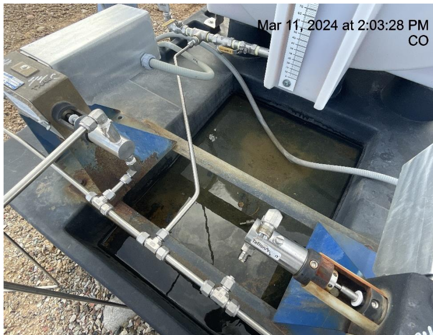
Photo # 9284 Chemical tank containment approximately 7/8 th full of fluid/failure to maintain chemical BMP/BMP insufficient to contain possible spill
