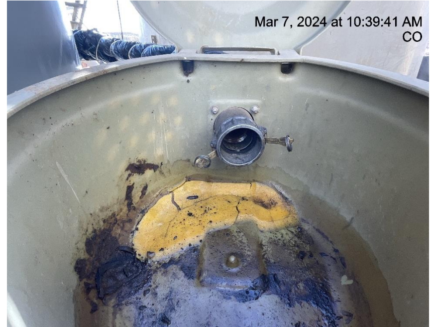
Photo # 9015 Open ended load line
