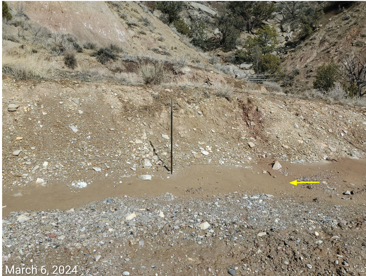
Photo 5: See comments under photo 4. Photo also shows sediment deposition due to erosion at the unstabilized slopes.
