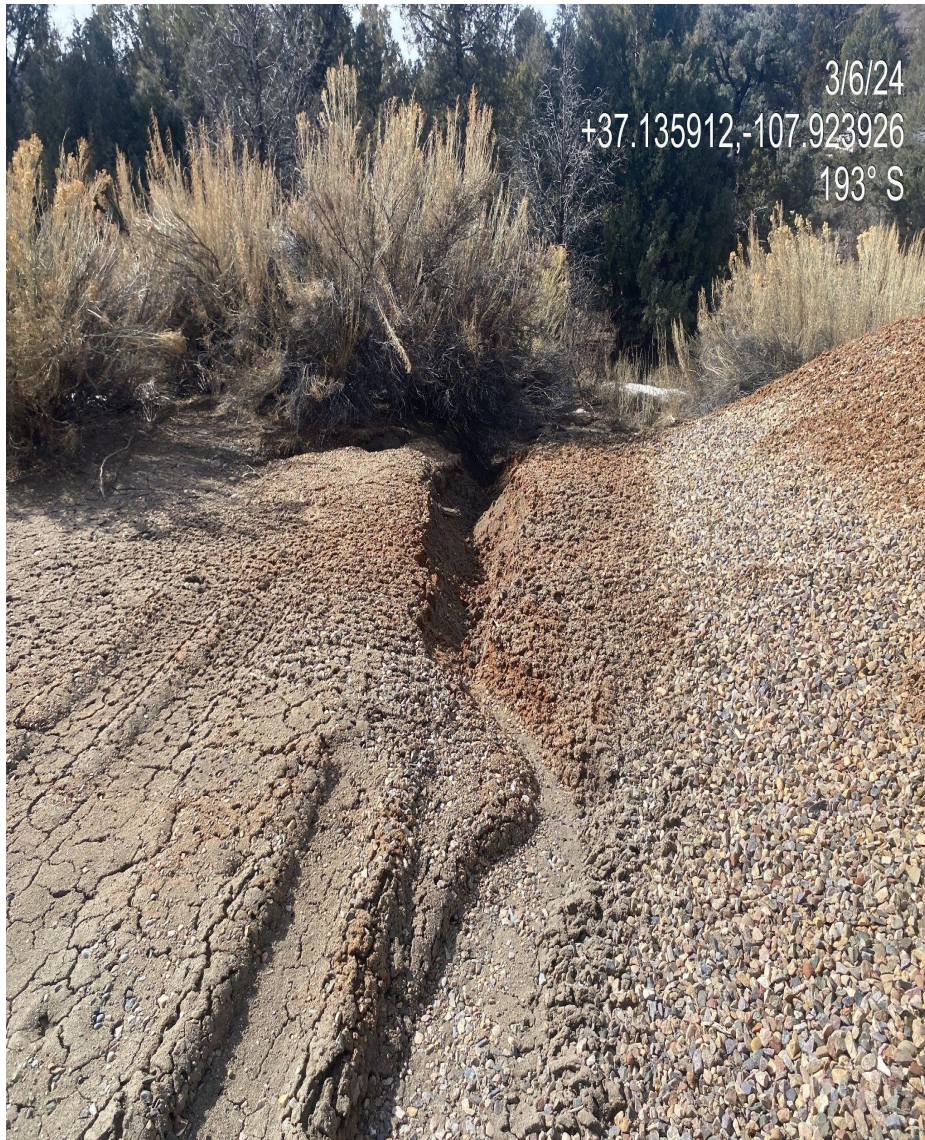
Photo 5. View of gully erosion forming on the western edge of the disturbance.
