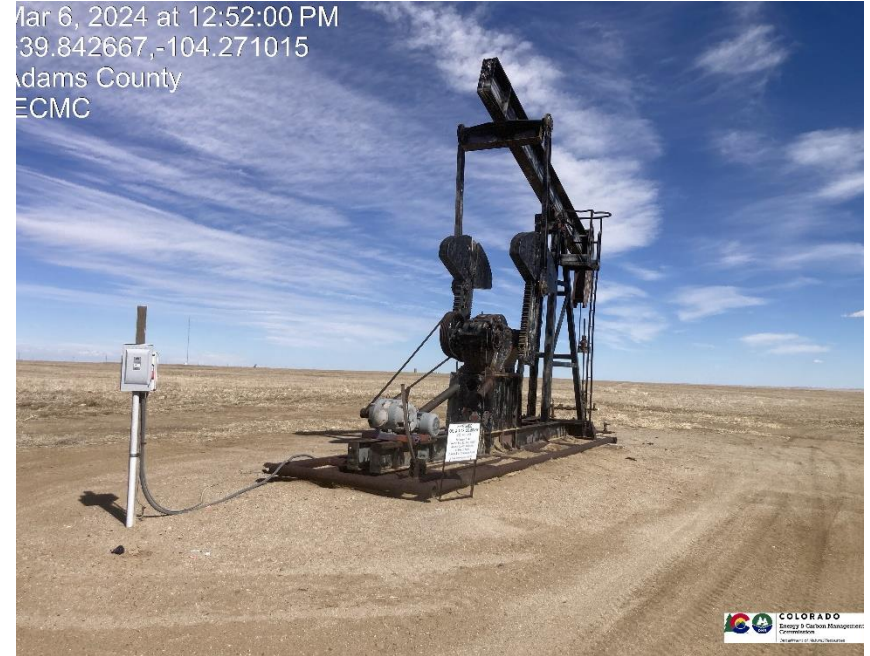
Pic 2 wellhead / pump jack
