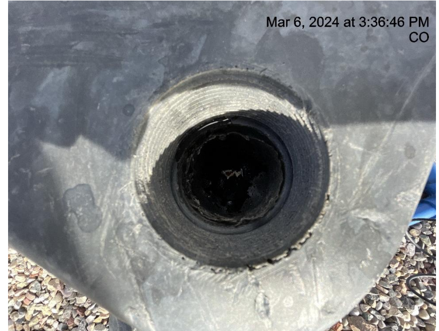
Photo # 8546 Chemical containment approximately 3/4 full of fluid/failure to maintain chemical BMP/BMP insufficient to contain possible spill.
