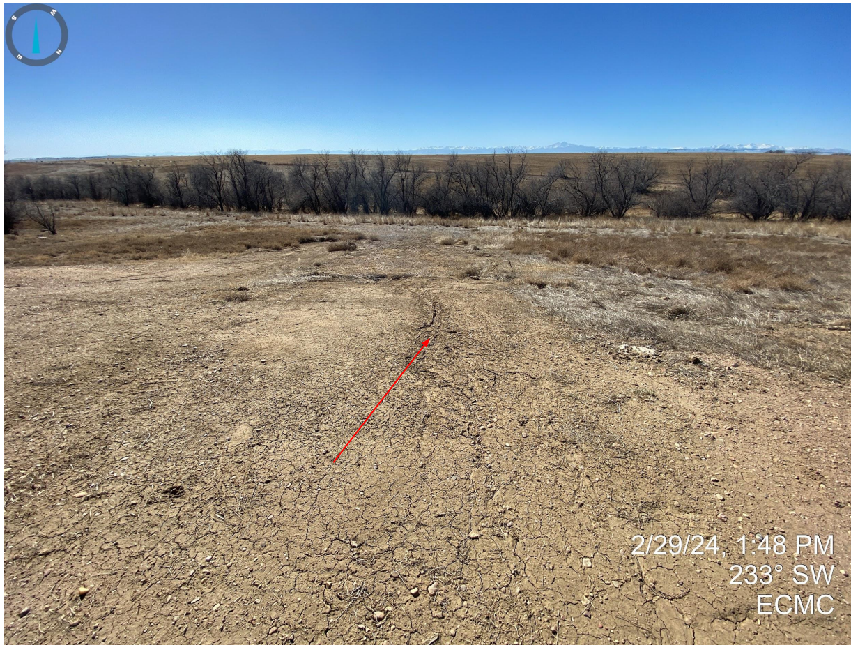
Photo 9. Western portion of location. Erosion degradation appears to have been repaired previously; no apparent stormwater control measures/BMPs observed to manage stormwater runoff. Bare soils require additional reclamation activities to stabilize the soils.
