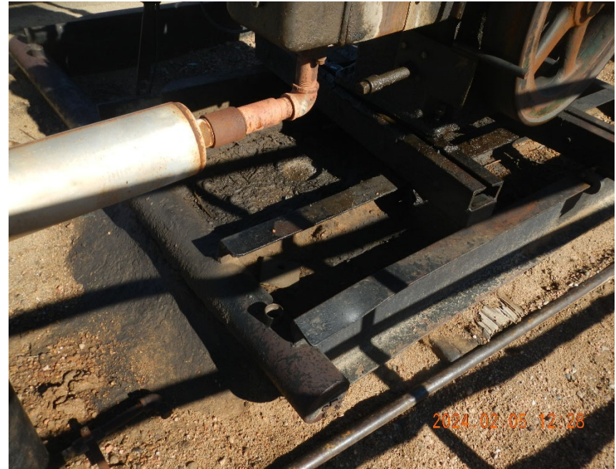
4. View of the base area around Pump Jack Prime Mover. Note stained soil under and around motor.
