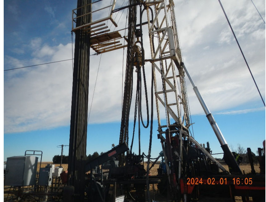
4. Power Swivel hung and running to drill the cement out of production casing.
