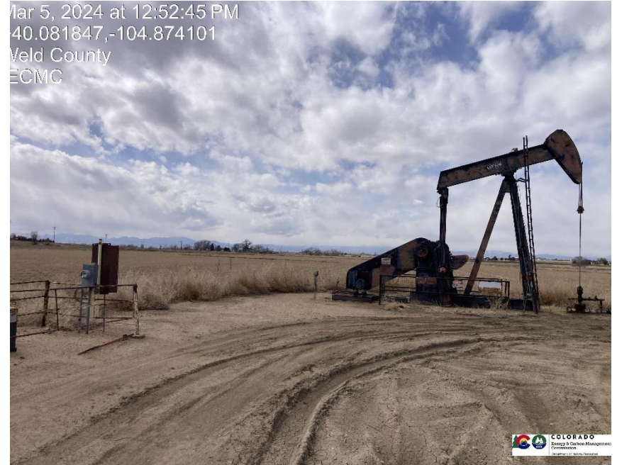
Pic 2 wellhead / pump jack
