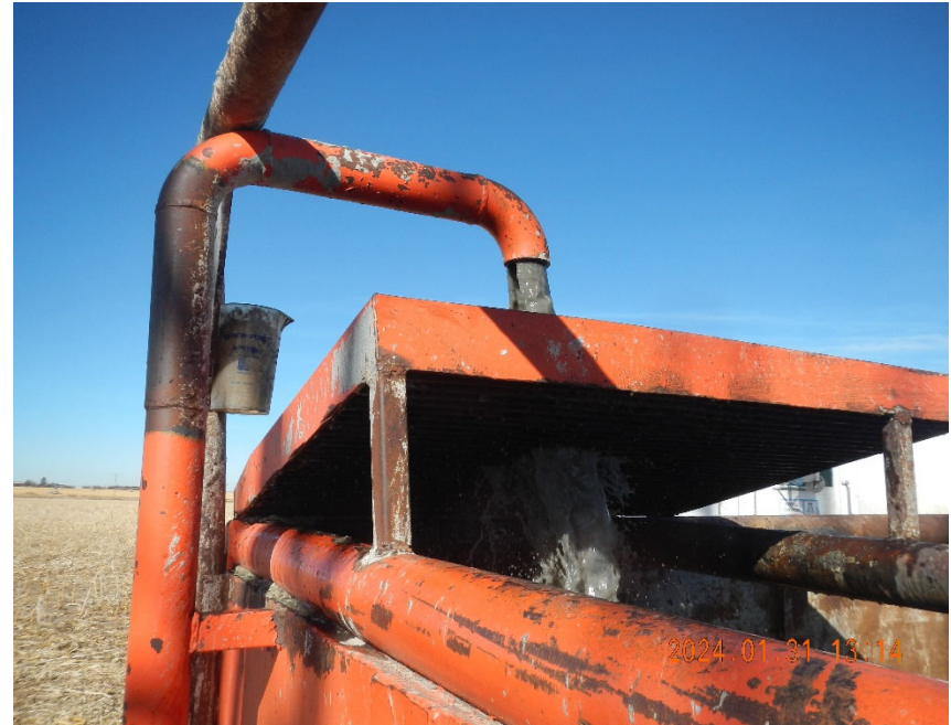
4. Returns to surface as well is circulated to clean up wellbore for cement work.
