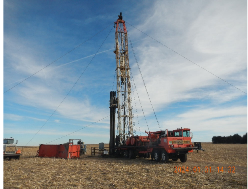
6. Work-over Rig rigged up on well.
