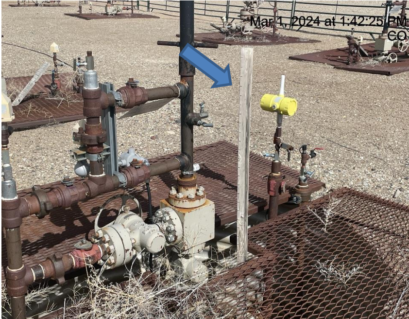
Photo # 8156 Wildlife egress on BAT 14B-17-07-95 well cellar not installed properly
