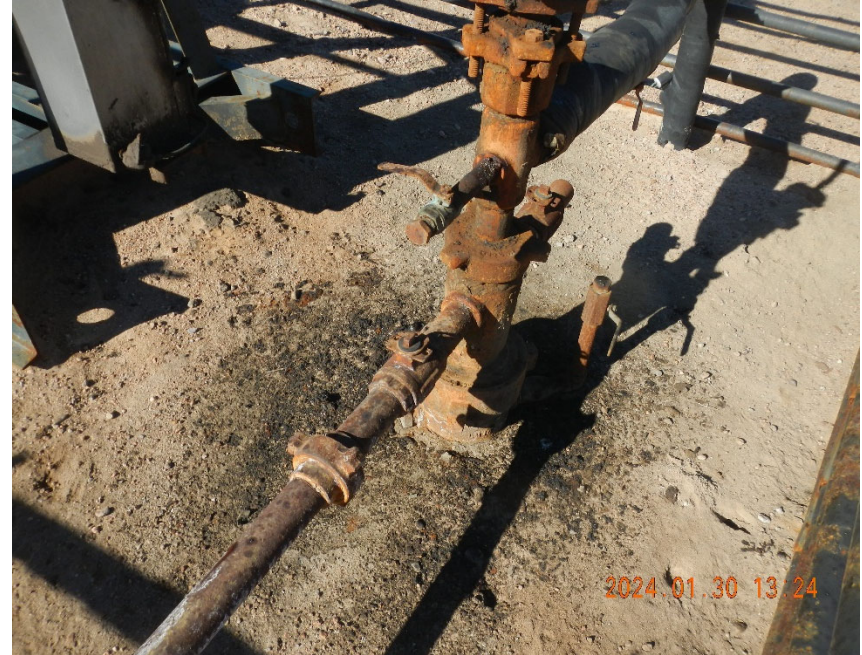
2. View of wellhead. Note staining around wellhead.
