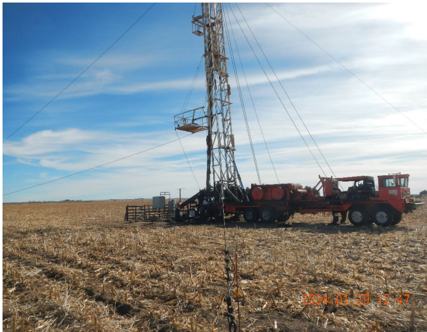
3. Work-over Rig rigged up over well.
