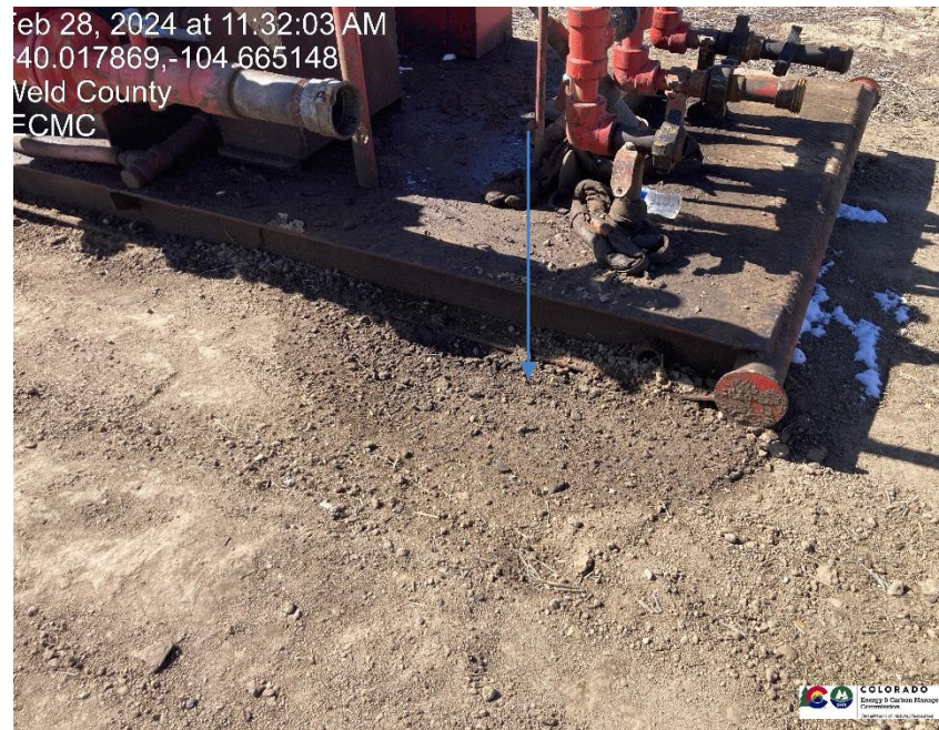
Pic 14 stained soil near tank
