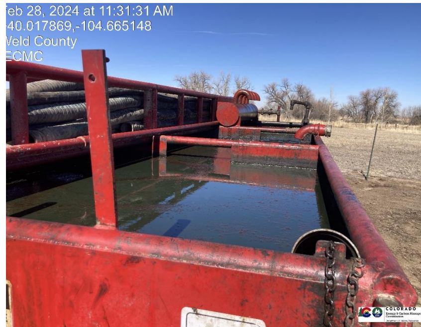
Pic 12 bird netting is not in place on open top tank.
