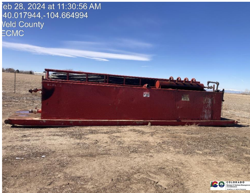
Pic 11 tank on location needs to be removed, wellsite activities have been completed, no stormwater containment.
