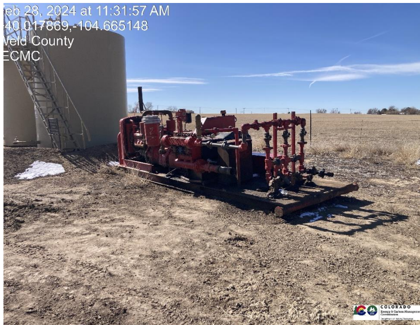
Pic 13 rig tank, no stormwater containment.
