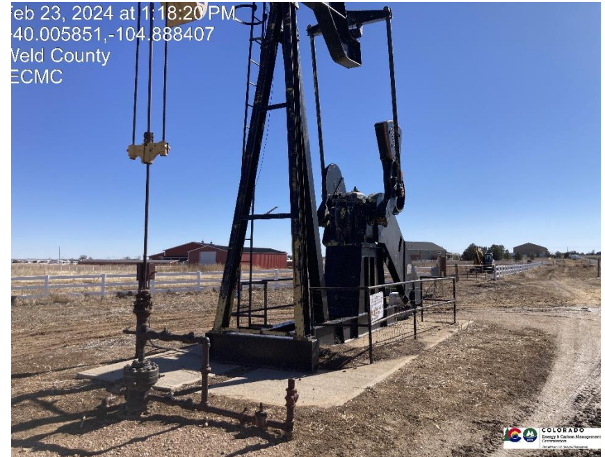
Pic 2 Pump jack / wellhead
