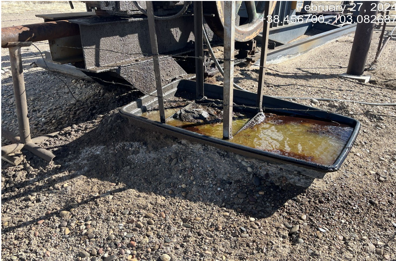
Photo 6. There is oily fluid in the containment next to the pump jack. Oily fluid has spilled onto the ground and needs to be cleaned up. Previous corrective action was not completed. Netting must be installed to prevent wildlife entry.
