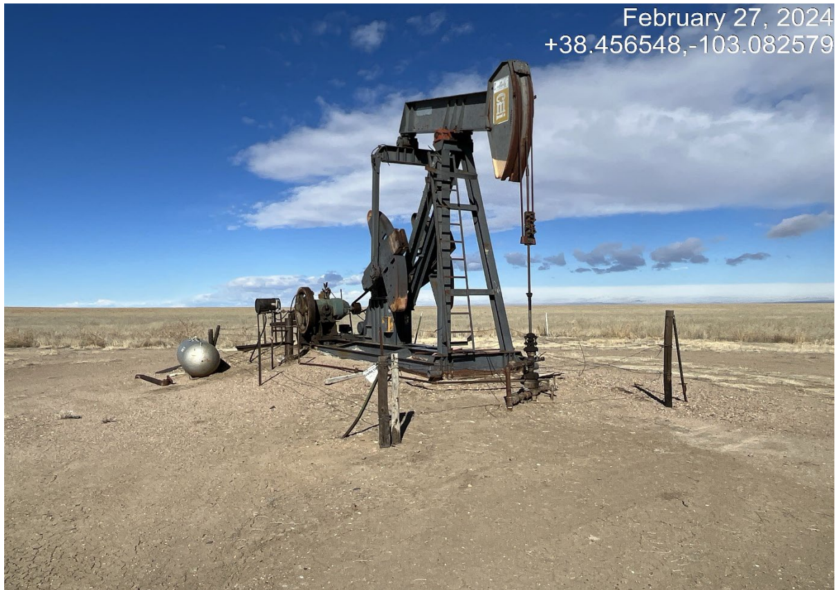
Photo 5. Facing northwest toward the wellsite. The fence around the pumpjack is in disrepair and won't prevent livestock entry.
