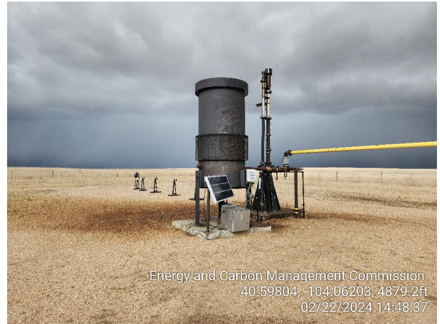
Photo 6 – Flare and ECD – Stained Soil
