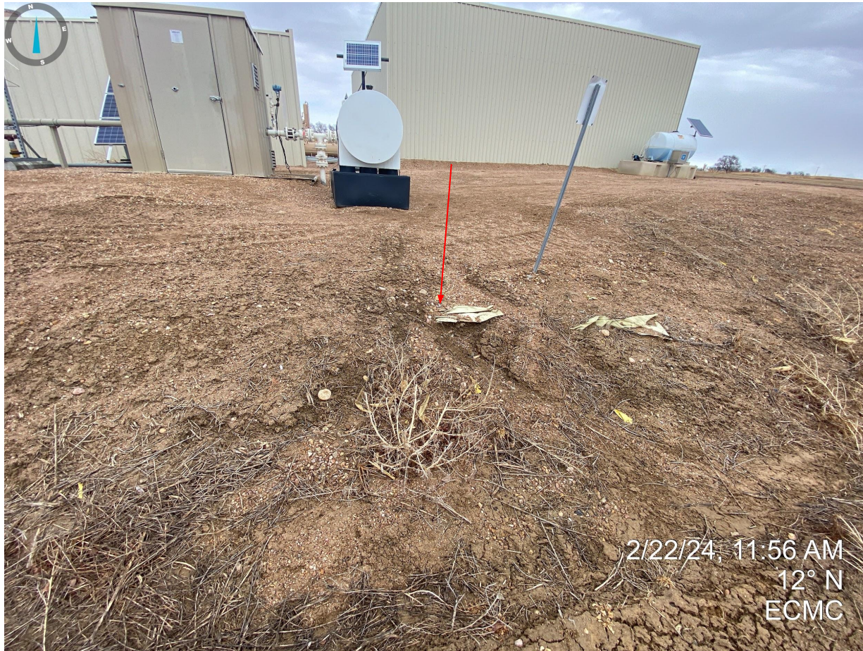
Photo 12. Erosion degradation occurring on the southern side of the production areas.
