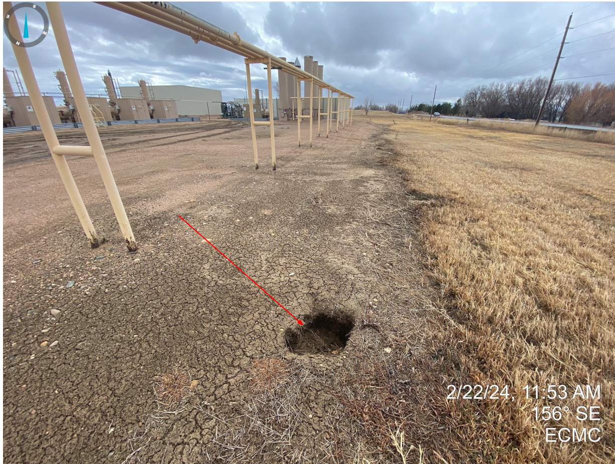
Photo 8. Hole/subsidence observed on the western side of the production areas (south of tank battery).
