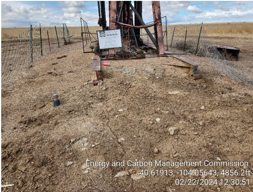
Photo 3 – Wellhead appears to have been Cut and Capped
