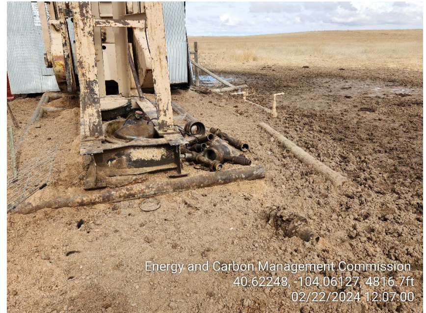
Photo 10 – Unused Wellhead Parts
