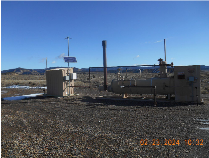
Separator and meter housing
