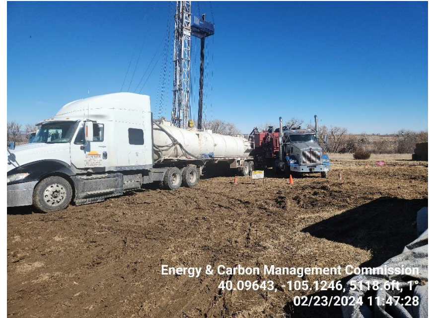
Photo 4 Fresh water transport & Axis Cement pump truck.
