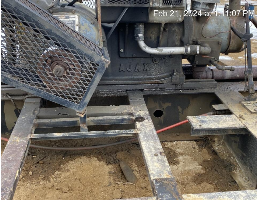
Equipment leaks and stained soil
