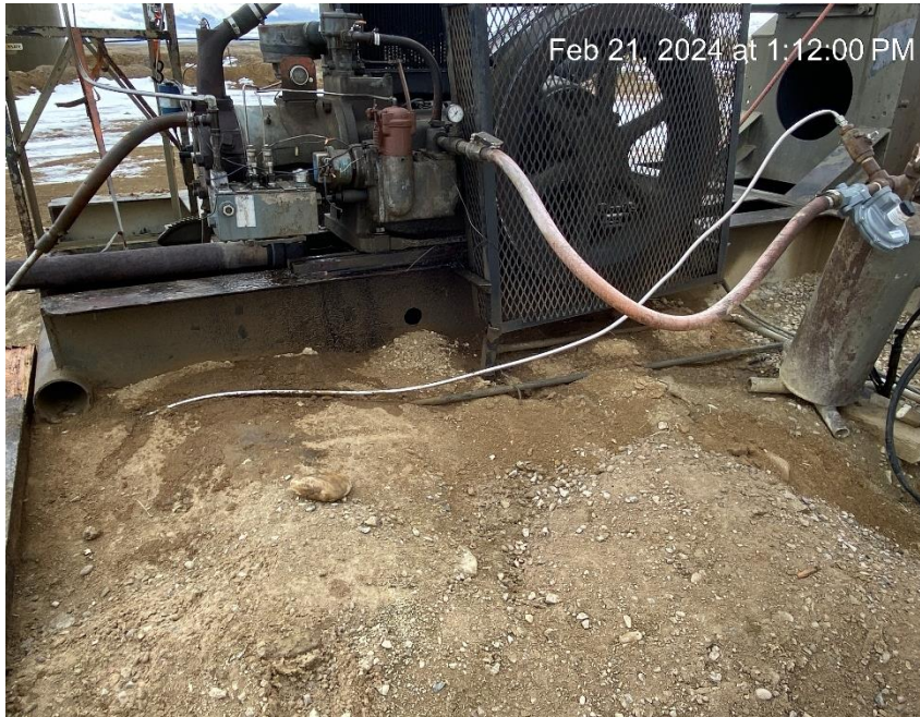
Leaking equipment and stained soil
