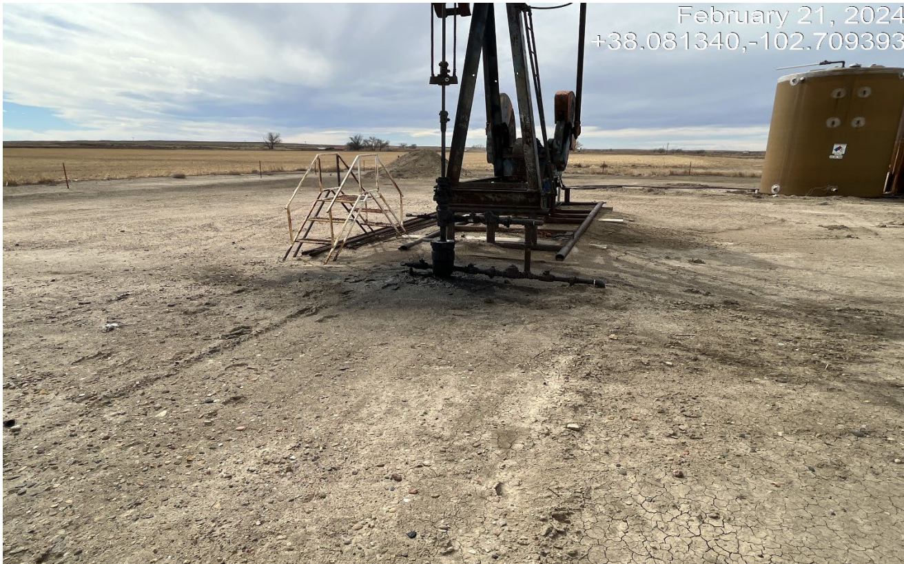
Photo 5. There is oil that has leak and sprayed out of the wellhead that needs to be cleaned up.
