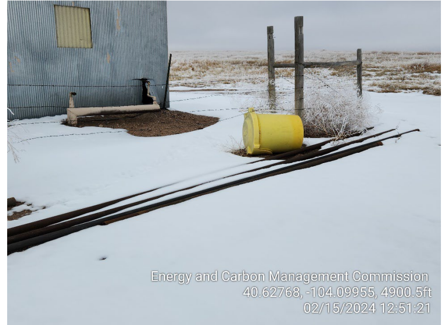
Photo 2 – Unused Tubing and Loadline Bucket
