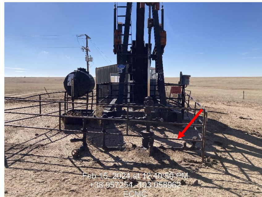
Photo 2 – Wellhead with oil staining
