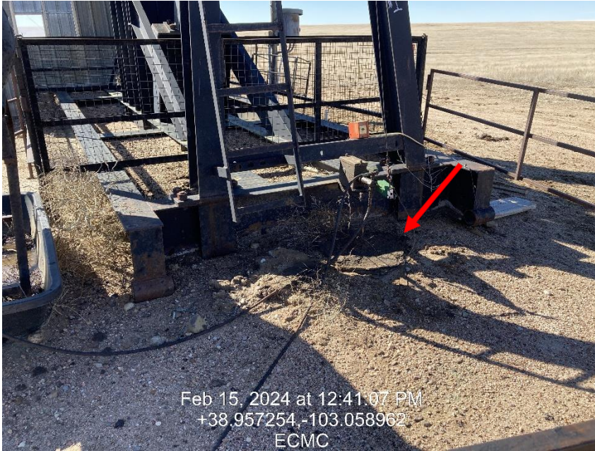
Photo 3 – Oil Staining at pumping unit base
