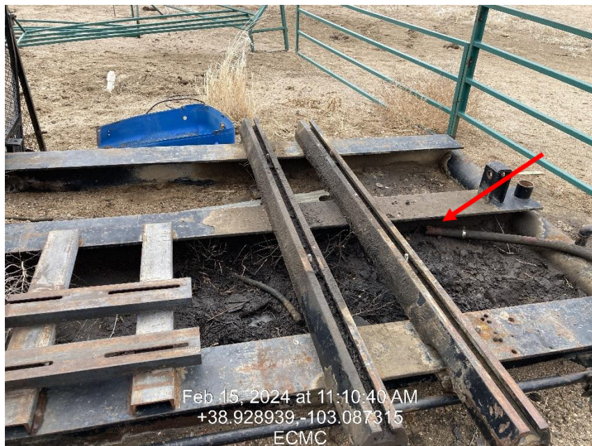
Photo 7 – Oil stained soils, Pumping Unit frame
