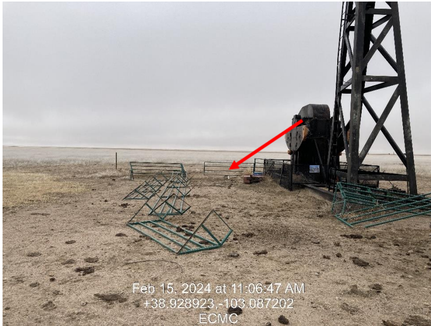
Photo 3 – Machine Guarding not maintained.
