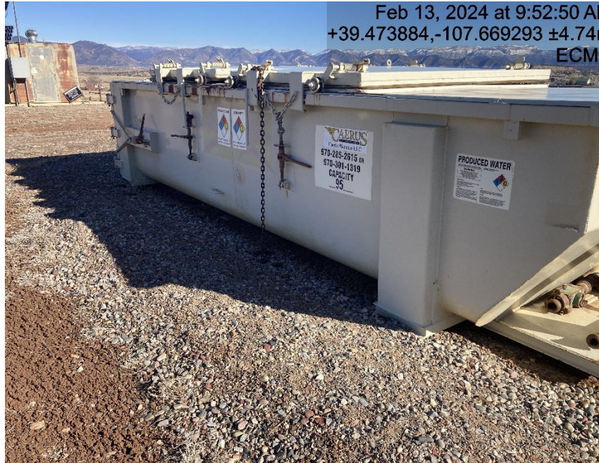
Lacking effective secondary containment
