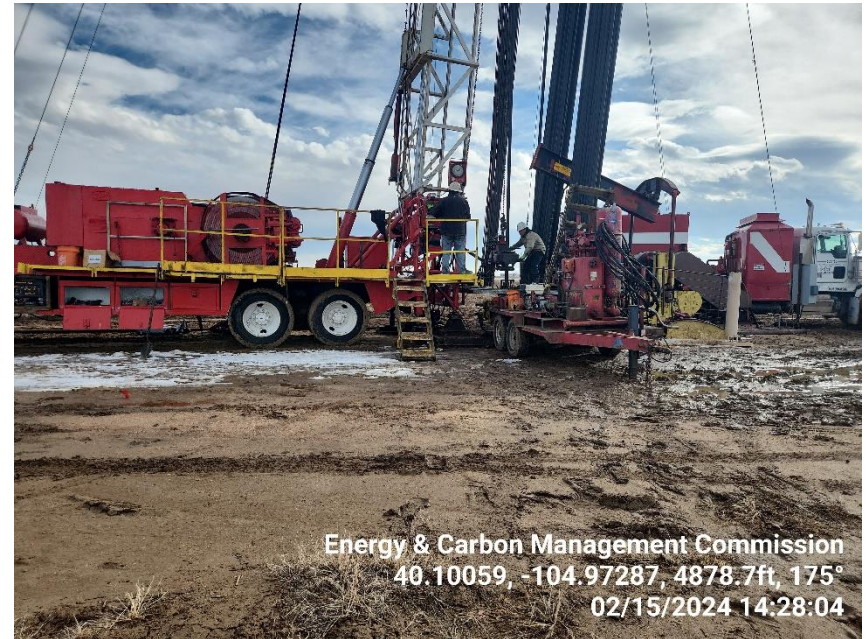
Photo 2 WO rig, accumulator trailers.
