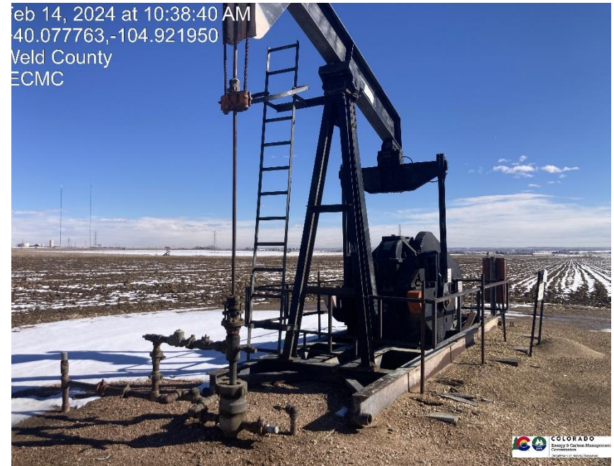
Pic 2 Pump jack / wellhead
