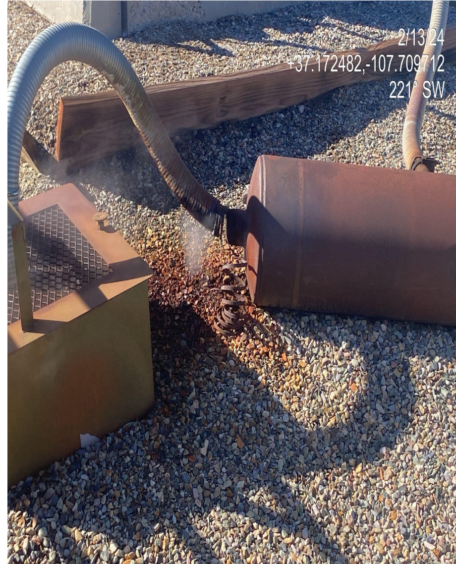
Photo 4. View of impacted materials at the well head and exhaust muffler.
