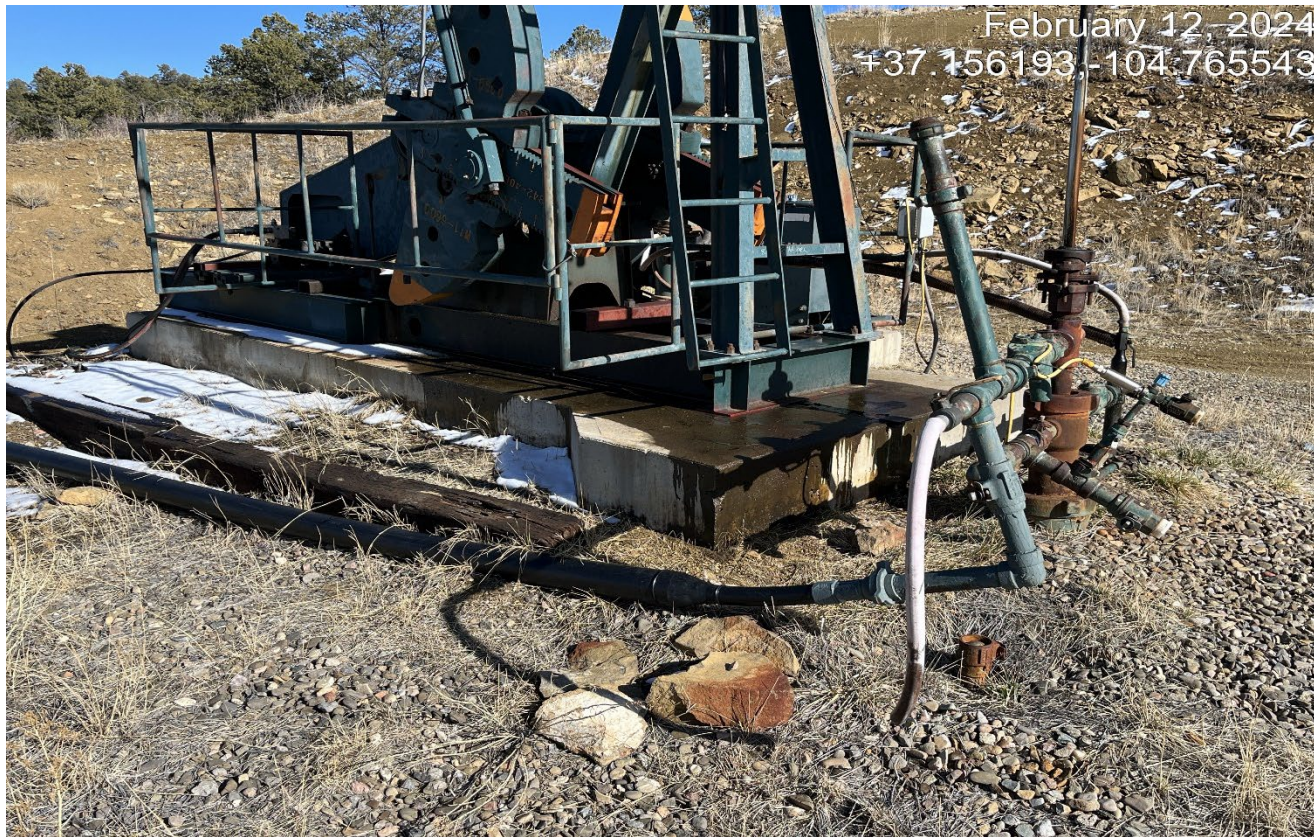
Photo 3. There is oily fluid leak at the pumpjack.
