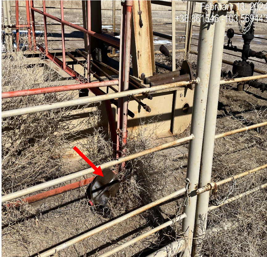
Photo 8. There is an oil filled milk jug that has tipped over and leaked oil onto the ground.
