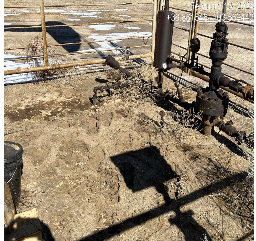
Photo 9. There is oily soils around the wellhead that need to be cleaned up.
