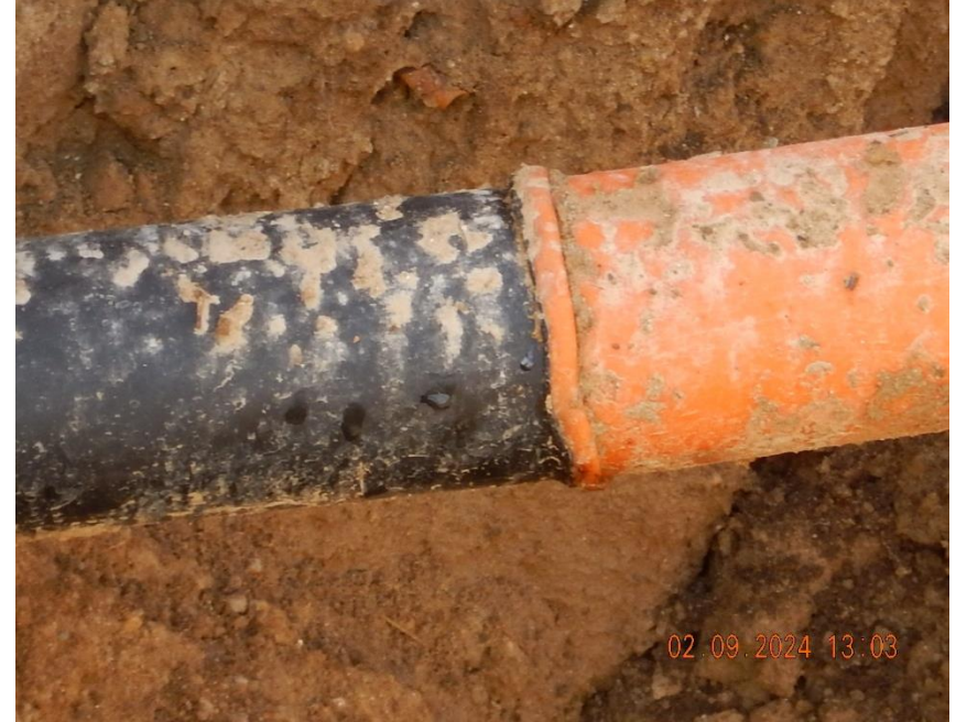
Close up view of butt end fusion weld; the orange weld bead is larger than the weld bead of the black pipe indicating improper pipe facing, heating and/ or alignment. The weld beads are not uniform around the pipe circumference.
