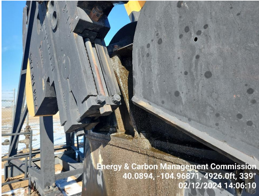
Photo 9 Gear box on the pump jack is leaking oil onto the ground.
