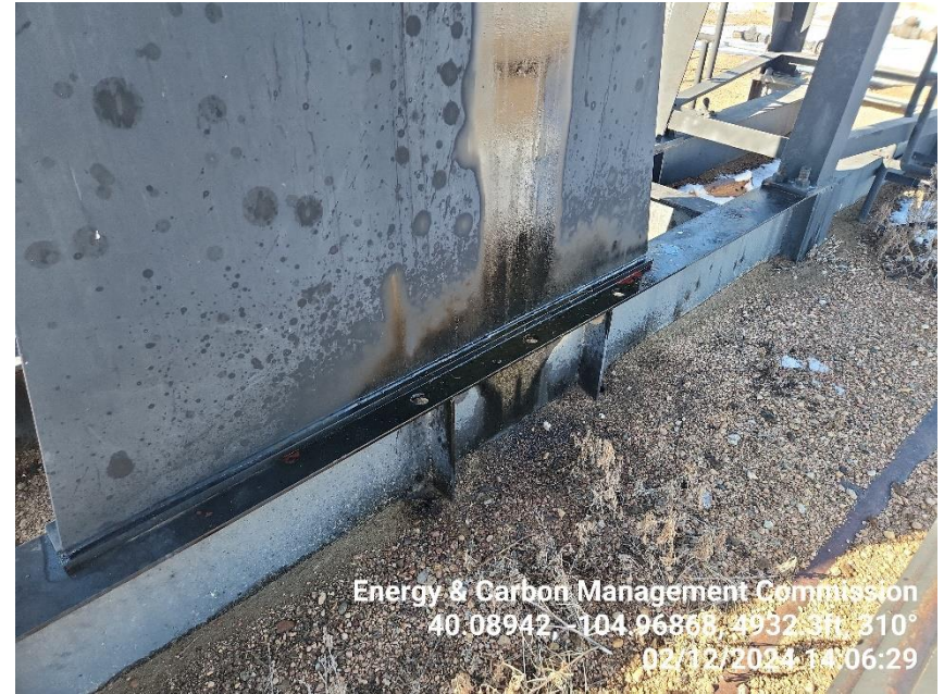
Photo 8 Gear box on the pump jack is leaking oil onto the ground..
