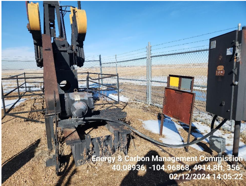
Photo 5 Prime Mover/Electric motor and electric panel.
