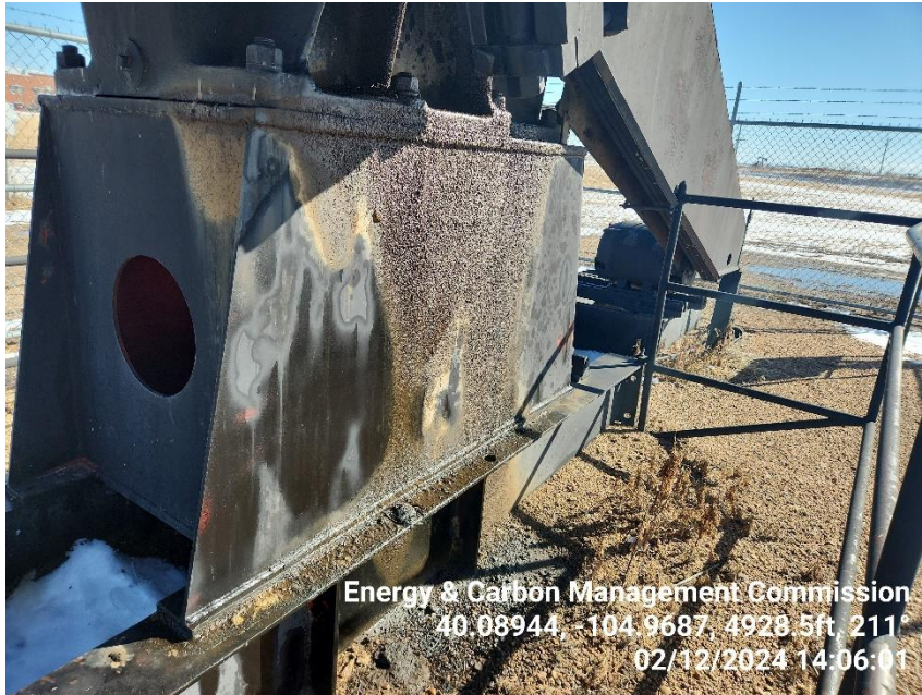
Photo 7 Gear box on the pump jack is leaking oil onto the ground.
