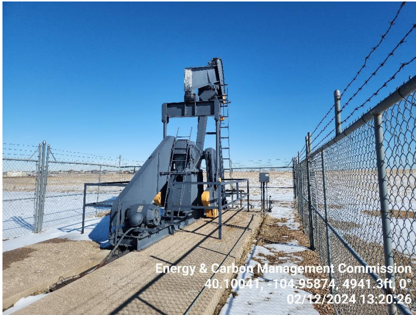
Photo 5 Prime Mover/Electric motor.
