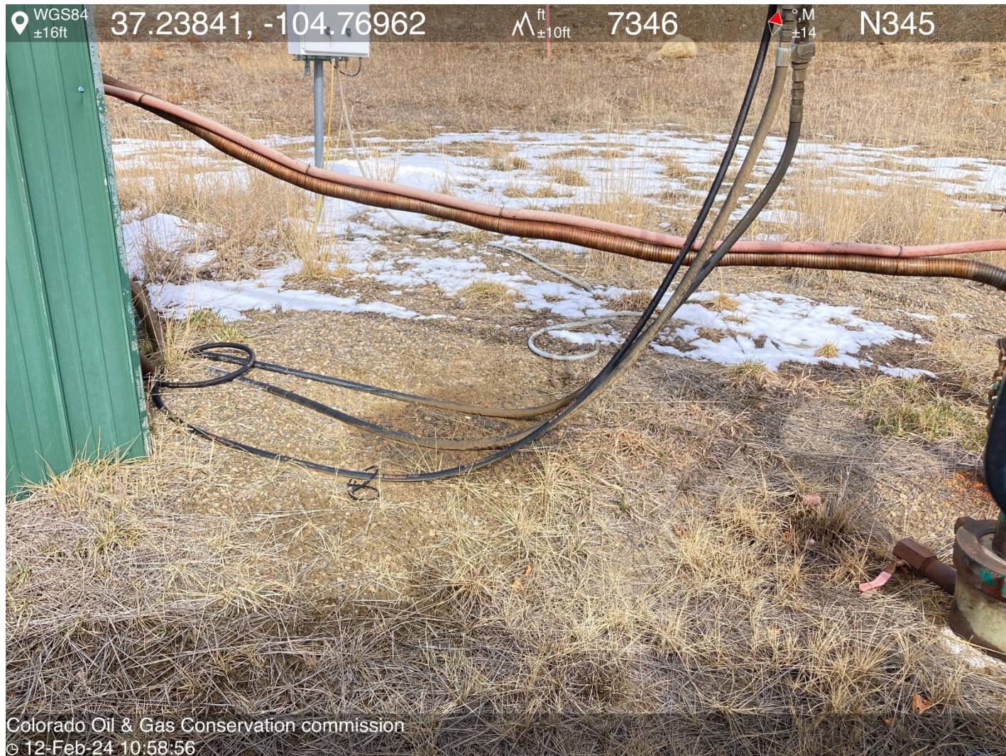
PHOTO 4: AREA OD IMPACTED OIL NEER WELLHEAD APPEARS TO BE LEAKING HYDRUALIC HOSES. Impacted soil identified at various locations through out location. CA DATE 3-12-2024.
