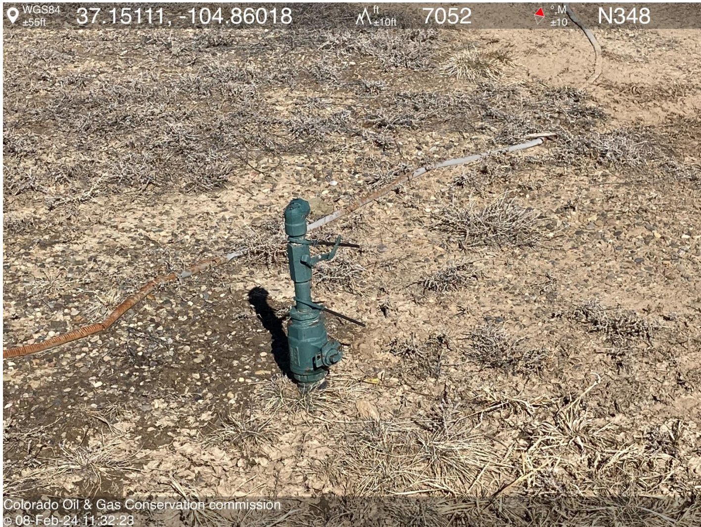
PHOTO 4: UNUSED RISER NOT MARKED. MARK OR REMOVE UNUSED RISER, COMPLY WITH RULE 606. CA DATE 3-8-2024.
