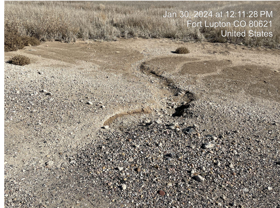
Photo 6. Photo taken of stormwater erosion on well pad perimeter. Photo taken facing south.
