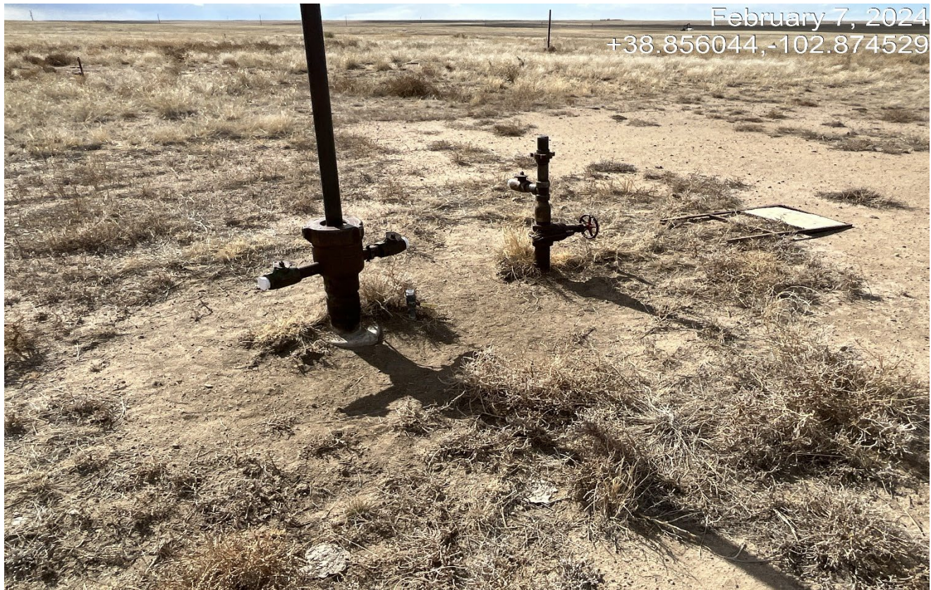
Photo 3. Facing toward the wellhead which has not produced for a very long time. Well sign has fallen over.
