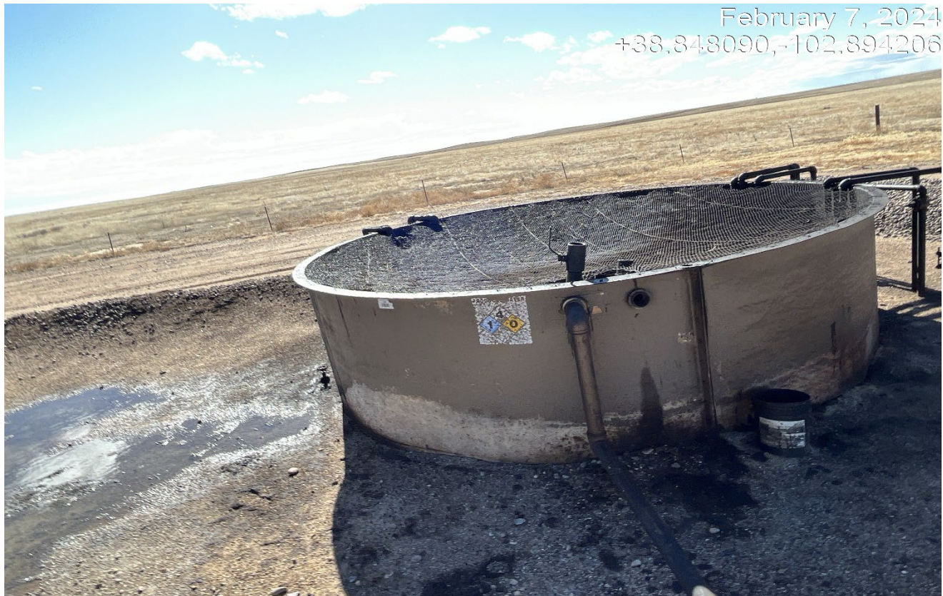
Photo 5. The open top tank is adequately netted. There was a spilled that occurred and oily soils need to be cleaned up.
