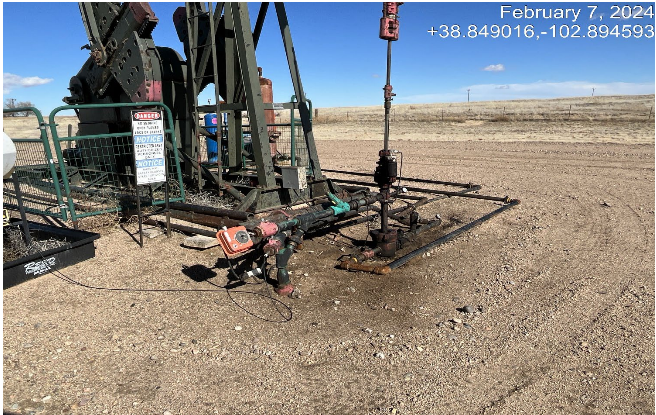
Photo 2. Facing toward the wellhead. There are stained soils at wellhead that should be cleaned up.
